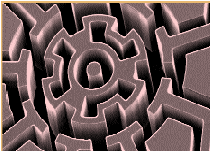
A wobble micromotor fabricated in a single crystal of silicon using a process combining deep reactive ion etching and wafer level silicon fusion bonding (Lucas Novasensor).
